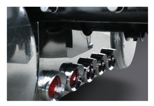
VU199002-5CR shown, includes lights and harness CHROME LIGHT BEZELS NOT INCLUDED WILL NOT WORK ON ALUMINUM FRAMES
